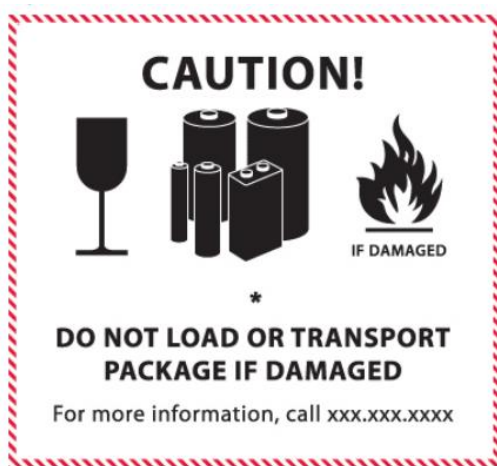
Figure 6: Transport and handling example label used in the aviation industry [20]
